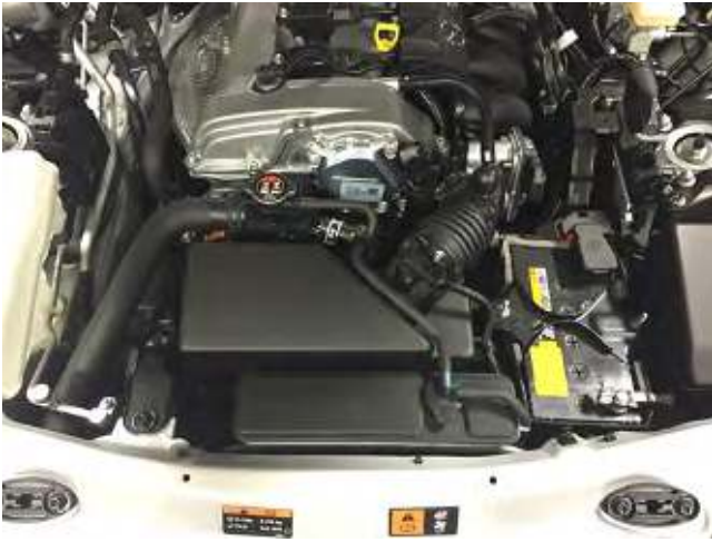
STOCK INTAKE INSTALLED
