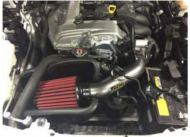
AEM INTAKE INSTALLED
